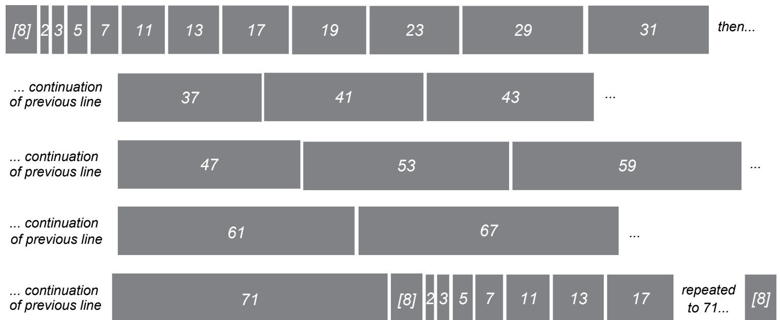
Prime numbers from 2 to 71 (to be read as one continuous signal): In this diagram each prime number is represented by a dark bar of the appropriate length of time (in white) in FTUs, as indicated by the numbers; a single interval of time (again in white) separates the numbers; the entire set of prime numbers occurs twice; a signal of 8 FTUs occurs at the beginning and end and in the middle to separate the two sets of prime numbers. One FTU is about a tenth of a second.
